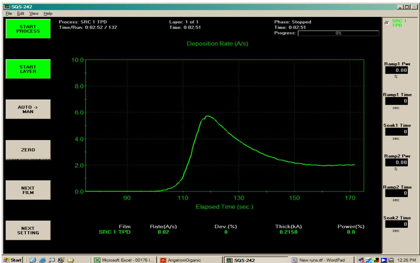
4 – If the power rose at a good speed and then the rate overshoot more than 50-60% and then came back down at a good speed then your I value is most likely very close to being right. You then have to increase the P value to drive the system both up and down faster to reduce the overshoot.
