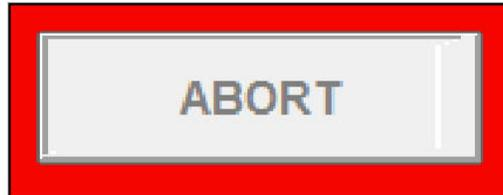
The abort button can be used to stop any automatic sequence. Note that this will close all valves including the gate valve (where applicable), and stop any active deposition process. A confirmation dialog box will open if the button is clicked.
