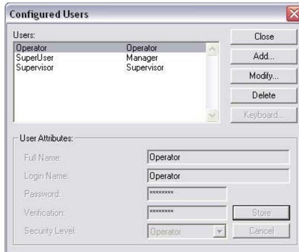
Supervisors have access to all the system controls, and they can change operator passwords and add other operators. There is a special password required to change supervisor passwords or add supervisors. There is no need to logout unless you are a Supervisor and you want to leave the machine to an operator. System Default User names/passwords are Operator/Operator and Supervisor/Supervisor. The login is case sensitive.
