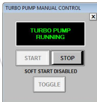
Soft Start can be enabled with the toggle button on the manual turbo pump control page. Toggle Soft Start and then start the pump. The turbo up to speed time delay setpoint is disabled when Soft Start is enabled as the pump takes more time to achieve full speed when the Soft Start function is enabled.
