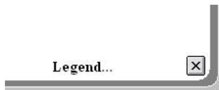
The X at the bottom right side of the screen closes all windows that are open if the user has been operating the system in manual and has a number of windows open clicking the X will close all windows.
