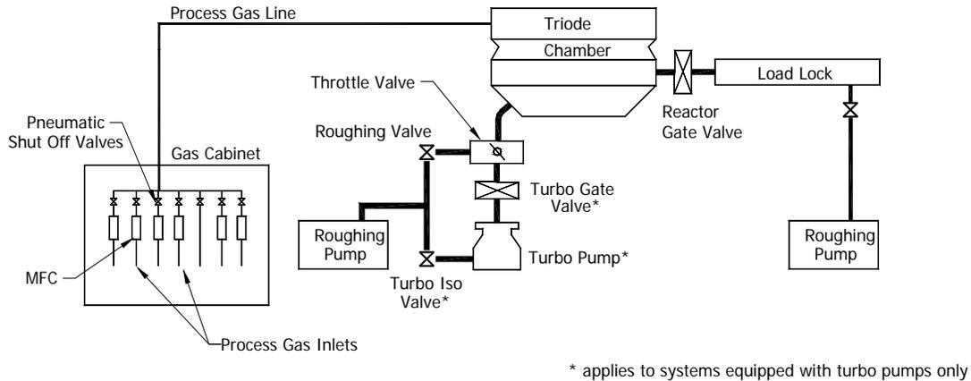
Figure 6. - Vacuum Schematic
