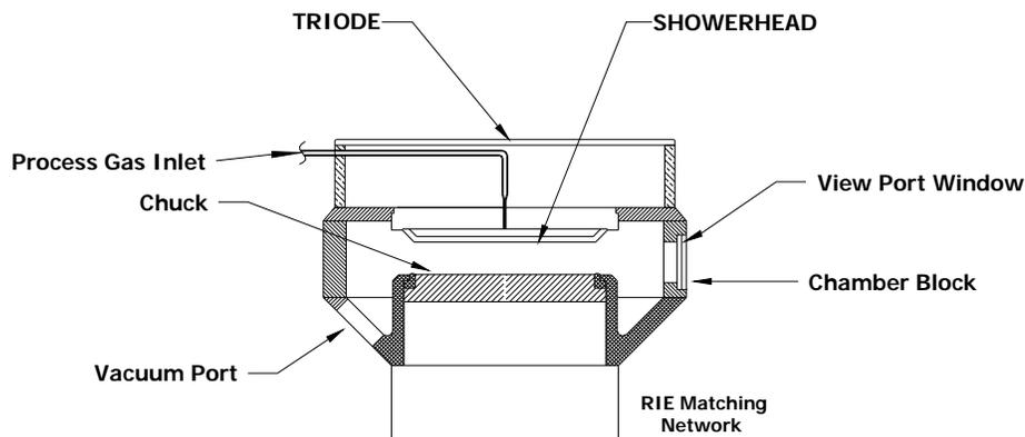
Figure 2. - Overall Process Chamber w/ TRIODE
